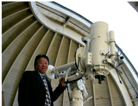
Dr T Ulaanbaatar with a 20 cm Maksutov telescope used for teaching astronomy at the National University. The telescope is on the roof of the Department of Geophysics in Ulaanbaatar
