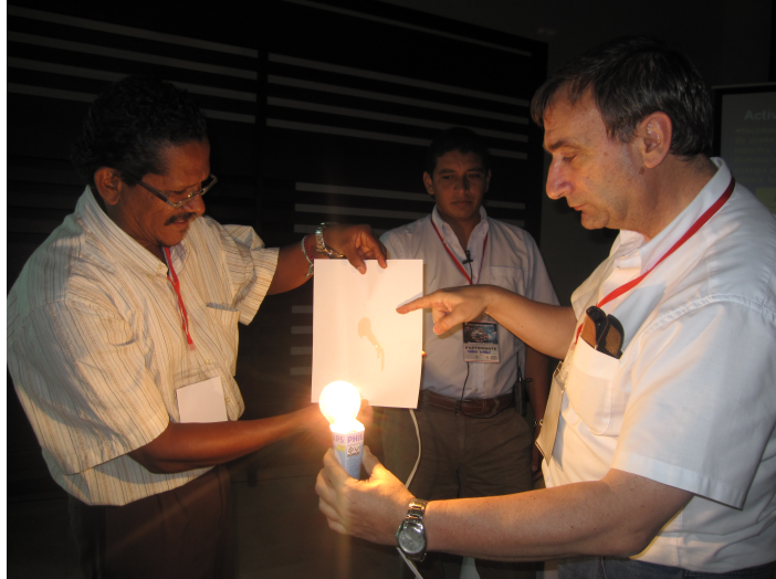
Students in Nicaragua performing the Bunsen grease spot experiment to compare the luminosity of two light sources
