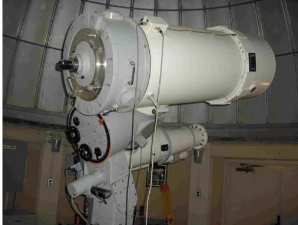
Figure 3 The 45 cm double telescope (non-operational)
