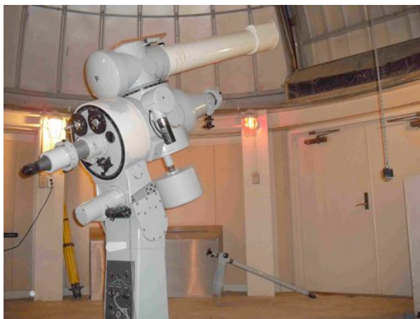
Figure 2 The 15 cm, F/15 Zeiss telescope (operational)
