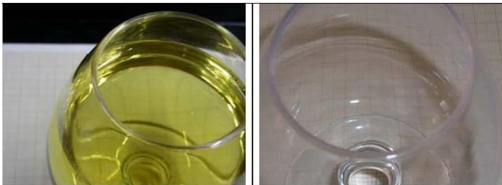
Fig. 2a and 2b: We only can see the distortion of the graph paper if the glass is full.
