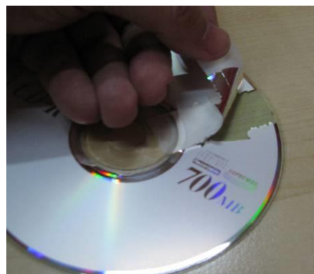
Fig. 6b: Removing the metal layer of the CD, with tape.
